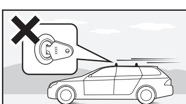
(EN) Always remove the key from the lock before driving. An inserted key may result in accidental openings and consequent load losses, causing damages and wounds, or even death, to those around you.
