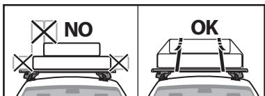
(EN) Load must be uniformly distributed with the lowest possible center of gravity. Load should not substantially extend beyond the loading surface of the roof rack. Ensure load stays within the perimeter delimited by the rack feet attached to the rails.
