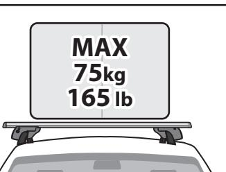
(EN) Do not exceed the maximum load specified for the roof rack, accessory rack or the maximum load recommended by the vehicle manufacturer. **Max roof load = weight of the complete roof rack system + weight of the load**
